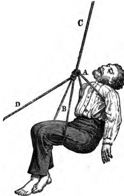
A. The arm loop. B. The leg loop. C. The hauling part. D. The guy.
