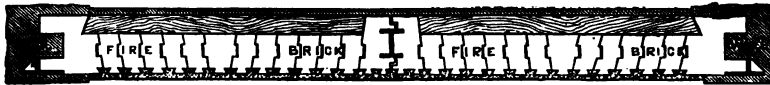
Section of Floor for Public Buildings, Mansions, &c. Joists and Boarded Floor on Patent Floor.
